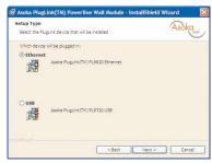
5. It is now time to connect your Asoka™ PlugLink™ device. Plug the PL9620-ETH into an AC outlet (no power strip or extension cord). Plug the supplied Ethernet cable into the PL9620-ETH and the Ethernet card on your PC. Click 'Finish' when the device is plugged in.
